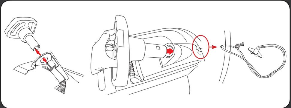
GB *Mounting/ Slide the steering wheel into the tube until it is completely fastened..*
